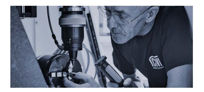
COVI's welding technologies encompass a range of unique technical advantages compared to traditional welding, MIG/MAG-, TIG- and arc welding. With a beam diameter down to 50 mµ, welding may be undertaken in areas that are difficult to access.
